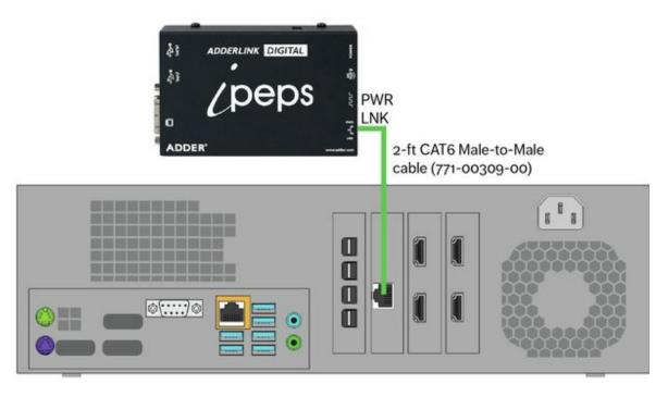
b. Connect the other end to the PWR-LNK port on the Adderlink ipeps unit of the IIC.
