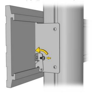
5. With a 5 mm hex wrench, loosen all 8 screws on the Display Height Brackets and set the distance between the tops of the Support Columns and the tops of the Display Height Brackets as follows:
