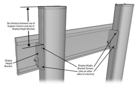
6. Tighten screws on Display Height Brackets.
