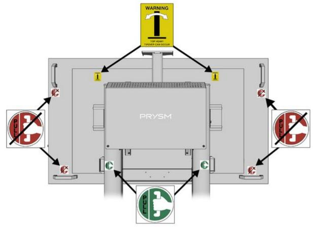
3. Apply the labels to the front of the left column and to the base of the Prysm Visual Workplace stand as shown below:
