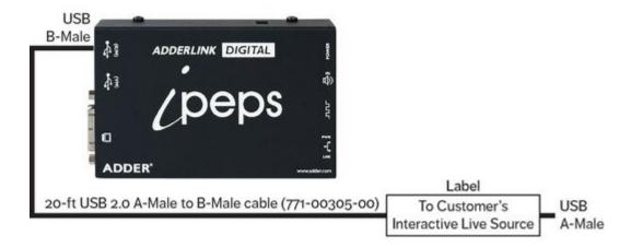
c. Mark the free end of this cable with a label indicating that it will be connected to the customer's Interactive Live Source (such as a laptop).
