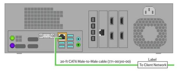
b. Mark the free end of this cable with a label to indicate that it will be connected to the client network.
