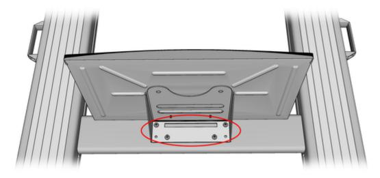
5. If you need to adjust the height of the keyboard shelf (recommended 10" down from the lowest edge of the display), loosen the two screws of the Center Support, slide the assembly up or down, then re-tighten the screws.
