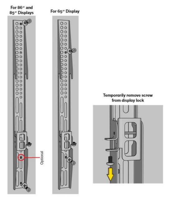
10. With a #2 Phillips screw driver, remove the screw on the Display Lock on both Display Hook Brackets, as shown above. Keep the screws to reinstall later.
