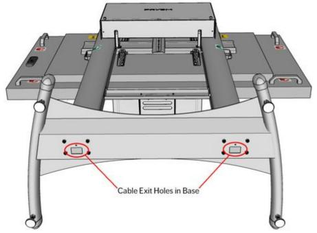
5. Once all cables are through, connect each cable at it's appropriate destination, including the power cable.
