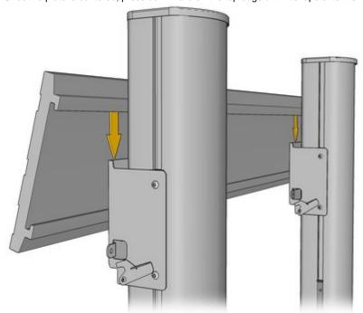
4. Rotate each Display Support Plate Lock back into position and reinstall the screws with a #2 screw driver.
